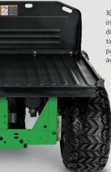
16.4 (.46 cu. m) cubic foot capacity reinforced box includes a gas-assist shock for easier lifting and dumping, pick-up style tailgate, 20 integrated tie-down points, and removable composite side panels and tailgate for flatbed operation. Also available: A factory-installed spray-on bedliner.
