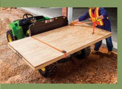
Composite sides can be removed in minutes, to convert the box to a flat-bed mode that's perfect for carrying large, awkward loads like plywood sheets, bales of hav, tables and more
