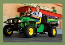
With a four-wheel suspension with coil over shock, triplerate adjustable springs the TX offers a smooth ride no matter what you haul
