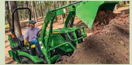
120R QUIK-PARK™ Loader Option. 72-in. (1.8 m) lift height. 803 lbs (364 kg) of lift capacity. Tool-free removal and attachment.
