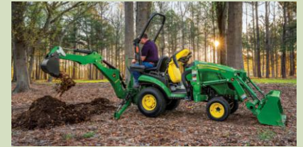
The 260B Backhoe Option. 8-ft., 8-in. (2.6 m) reach with a dig depth of almost 7 feet (2.1 m). Optional mechanical backhoe thumb is available to help lift debris.
